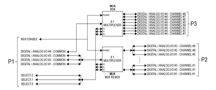
The I/O group width can easily be extended by operating several G-MUX devices in parallel. One G-MUX device can be the Master device (controlled via USB). The other devices can be controlled by the MUX Control signals which are available on P1 of the Master device (see section G-MUX usage examples for examples of how several G-MUX devices can be connected together).
