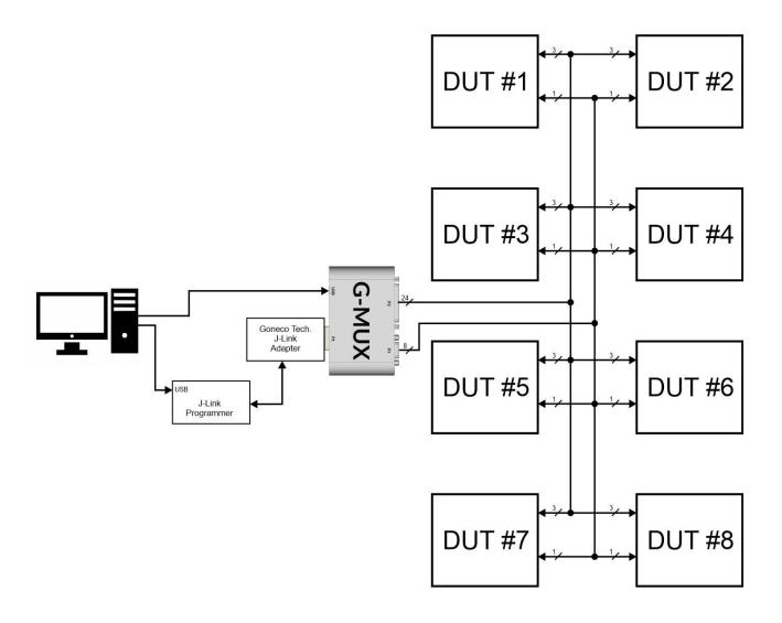
Note: The Goneco Technologies J-Link Adapter (Model Number JLA-2402) provides a 10 pin header which allows the connection of a standard 10 pin connector J-Link ribbon cable to the G-MUX I/Os. Click <a href="here">here</a> for a detailed description of this adapter.
