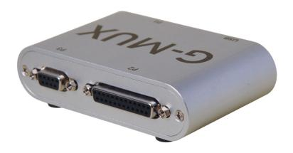
The Goneco Technologies G-MUX (Model Number GMX-2401) provides the ability to multiplex a group of four individual analog and/or digital signals to 1 of 8 output channels. This feature is particularly useful in such environments as production testing or production programming. The four individual signals can be used for both analog and digital signals, thus making the G-MUX useful for multiplexing analog signals as well as common serial protocol systems such as UART, SPI, and I2C.
